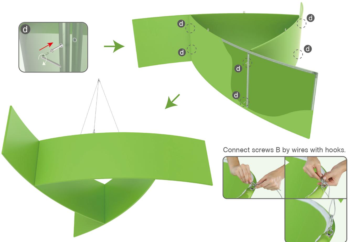
Connect screws B by wires with hooks.
